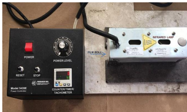
Figure M2-5. Photo of inline RTP system for roll-to-roll annealing features a multi-function controller and an IR lamp.
